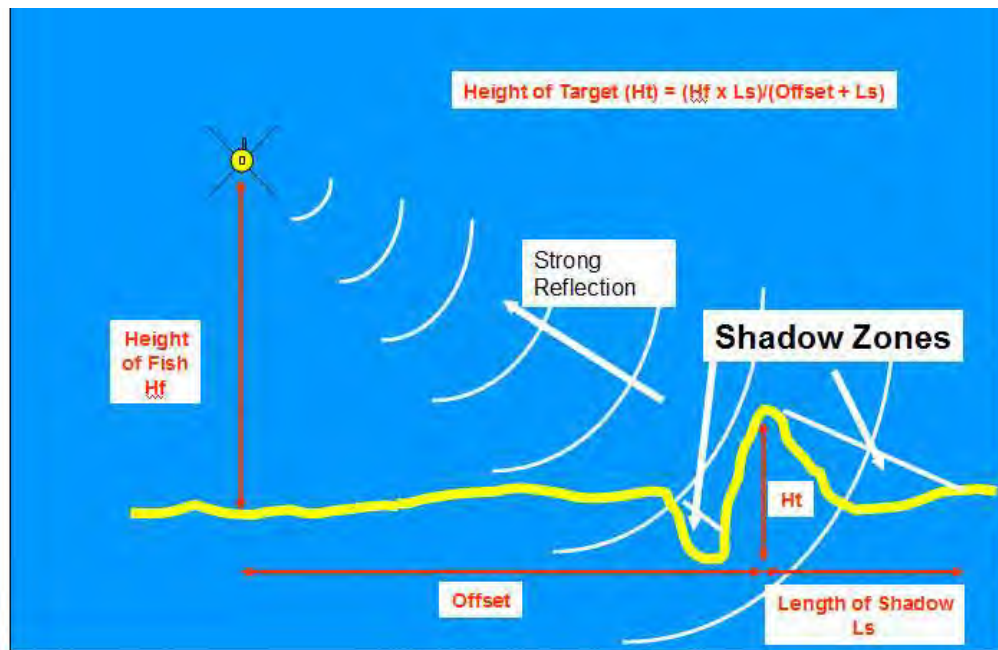
Figure Q-5. Side scan height and contact height computations (NOAA)
